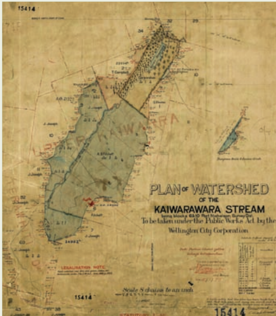
This plan of the Kaiwharawhara Stream watershed, dated 1901, shows the catchment land to be purchased (blue) in relation to the planned upper dam and reservoir.
