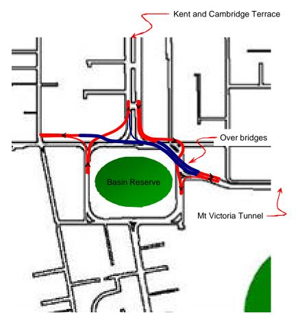
Figure 13.7: - Option B3 Alignment for Two Way Grade Separated Option at the Basin Reserve
