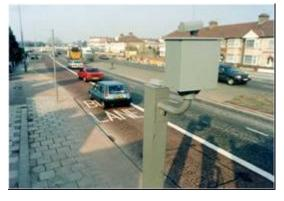
Figure 7.8: -CCTV Enforcement Camera
