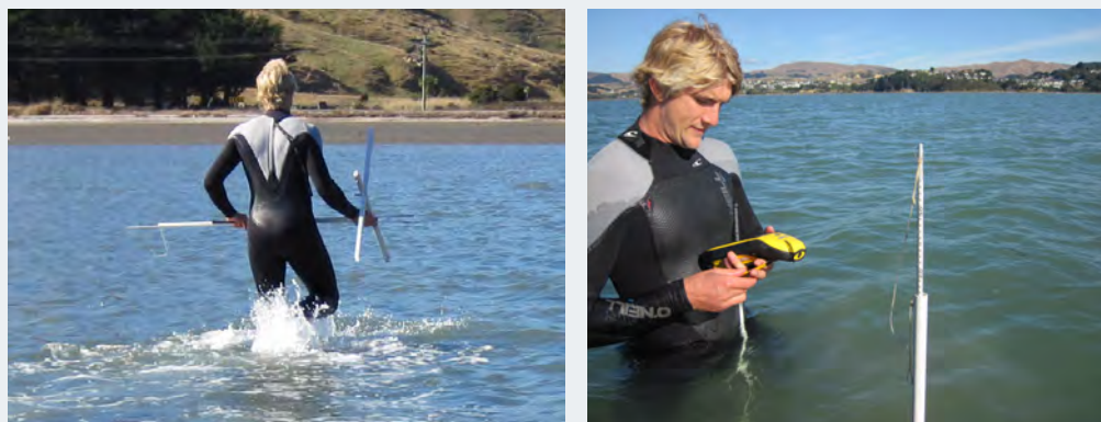
Measuring frame and probe used to measure shallow subtidal plates.
