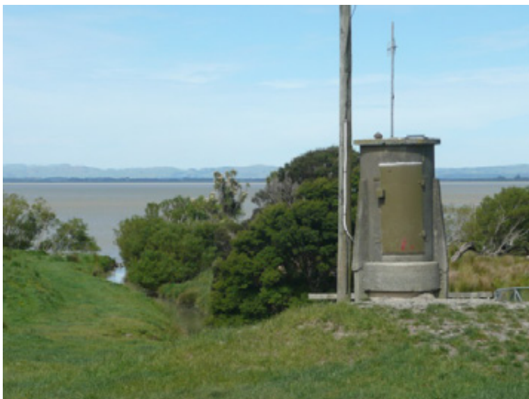
Figure 4.5: Burlings lake water level recorder located on the south western shore
