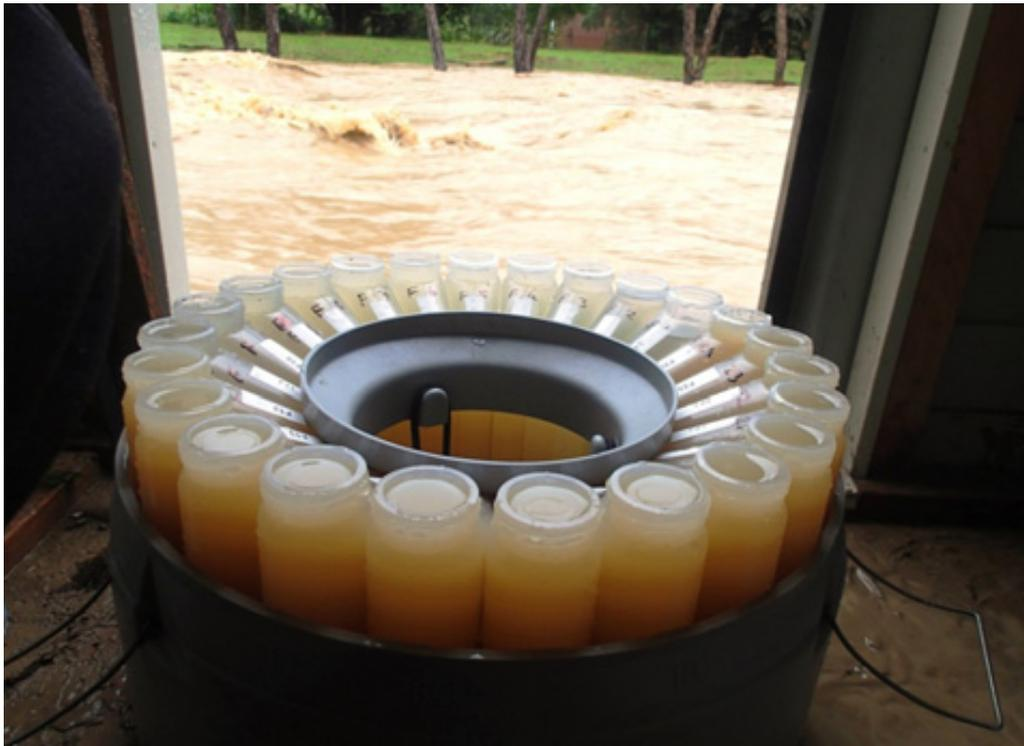
**Figure 2.5: Autosampler bottle carriage with 24 samples collected on 14 May 2015 at the Horokiri Stream monitoring site. This flood was a 10-year return period event for the Horokiri catchment**
