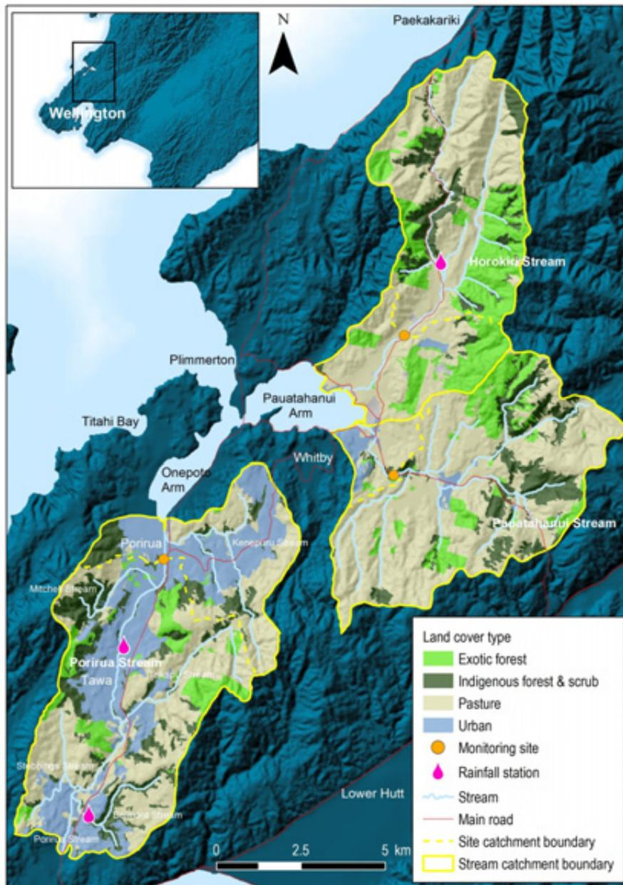
**Figure 2.1: Location of the three continuous turbidity monitoring sites in the Porirua Harbour catchment and the major land cover types within each catchment. Areas downstream of the dashed site catchment line are not captured by the monitoring site**
