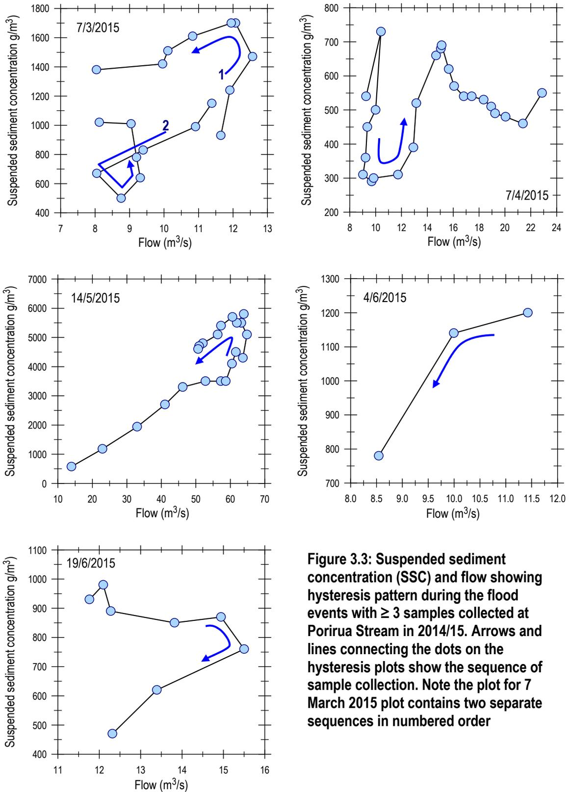
**Figure 3.3: Suspended sediment concentration (SSC) and flow showing hysteresis pattern during the flood events with  $\geq 3$  samples collected at Porirua Stream in 2014/15. Arrows and lines connecting the dots on the hysteresis plots show the sequence of sample collection. Note the plot for 7 March 2015 plot contains two separate sequences in numbered order**
