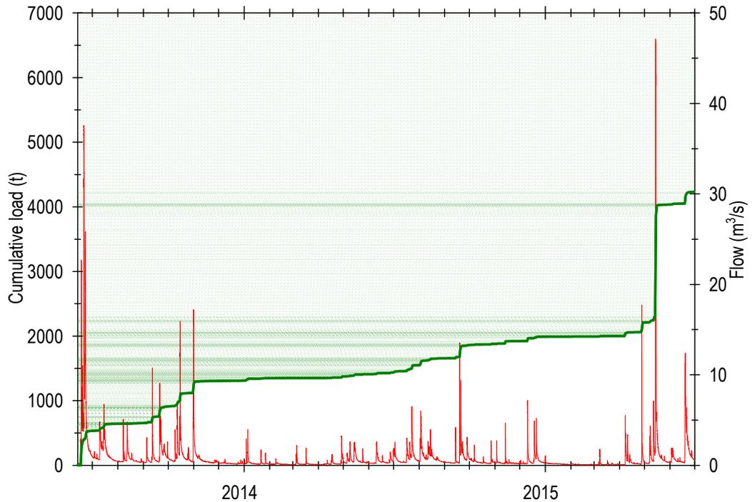
**Figure 3.14: Cumulative sediment load (green line) versus stream flow (red line) in the Pauatahanui Stream from 13 June 2013 to 30 June 2015**
