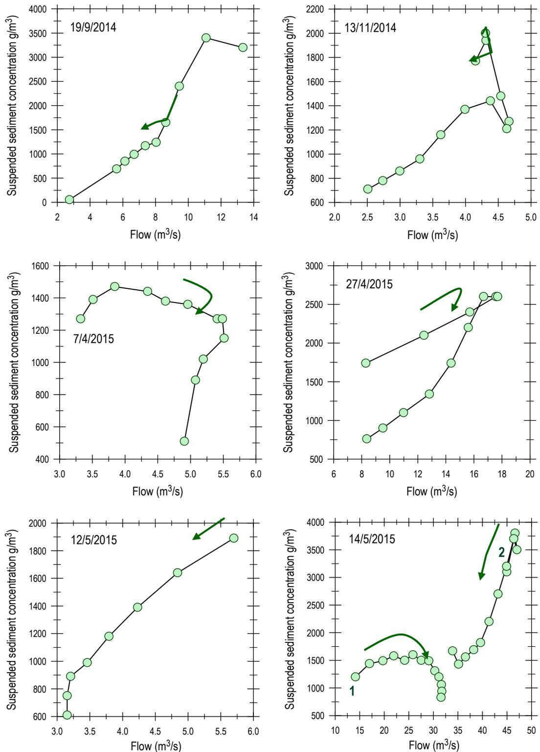
**Figure 3.13: SSC and flow showing hysteresis patterns during the flood events with  $\geq 3$  samples collected from Pauatahanui Stream in 2014/15. Arrows and lines connecting the dots on the hysteresis plots show the sequence of sample collection. Note the plot for 14 May 2015 contains two separate sequences (numbered in order) where samples were collected.**
