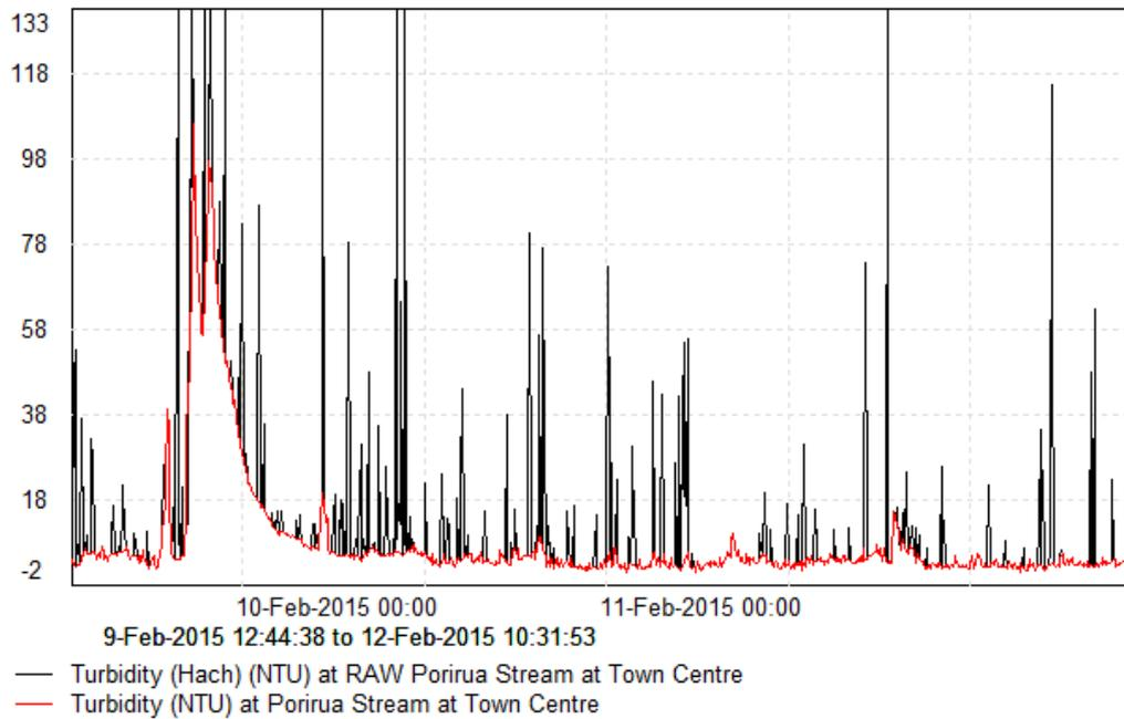
**Figure 2.6: Continuous turbidity record illustrating the raw (black) versus edited (red) turbidity data. The original raw turbidity trace shows the amount of noise that needs to be removed**
