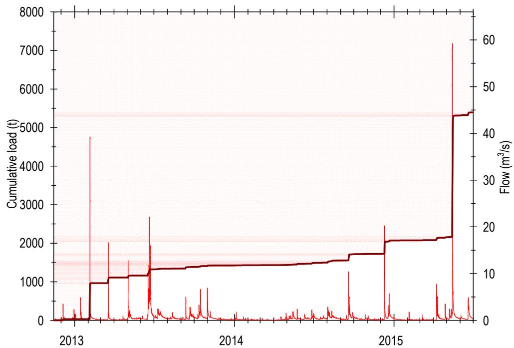
**Figure 3.9: Cumulative sediment load (maroon line) versus stream flow (red line) in the Horokiri Stream from 14 November 2012 to 30 June 2015**
