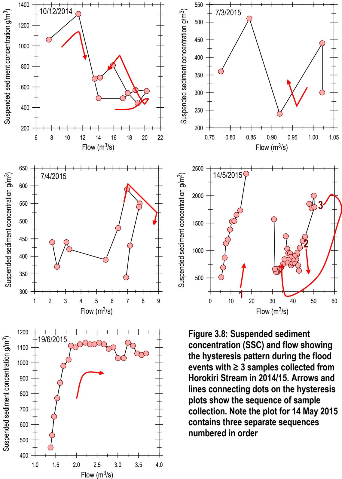
**Figure 3.8: Suspended sediment concentration (SSC) and flow showing the hysteresis pattern during the flood events with  $\geq 3$  samples collected from Horokiri Stream in 2014/15. Arrows and lines connecting dots on the hysteresis plots show the sequence of sample collection. Note the plot for 14 May 2015 contains three separate sequences numbered in order**
