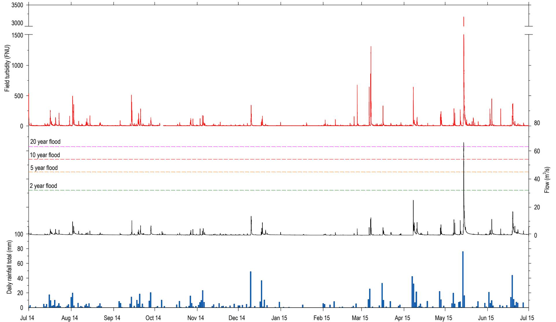
**Figure 3.1: Plots of (continuous) turbidity and flow at the Porirua Stream monitoring site and total daily rainfall at Seton Nossitor Park (or Tawa Pool where data missing) between 1 July 2014 and 30 June 2015**
