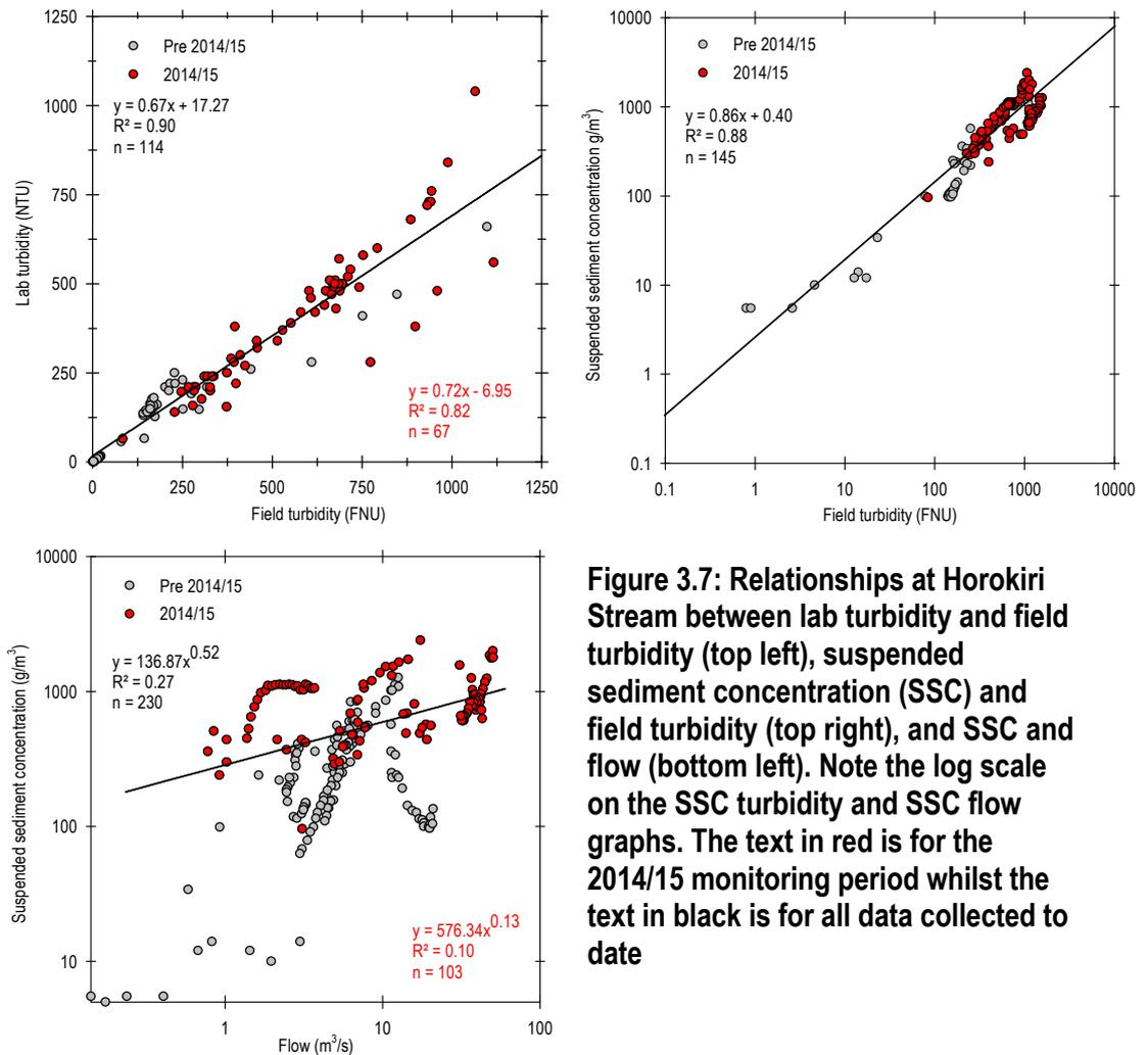
**Figure 3.7: Relationships at Horokiri Stream between lab turbidity and field turbidity (top left), suspended sediment concentration (SSC) and field turbidity (top right), and SSC and flow (bottom left). Note the log scale on the SSC turbidity and SSC flow graphs. The text in red is for the 2014/15 monitoring period whilst the text in black is for all data collected to date**
