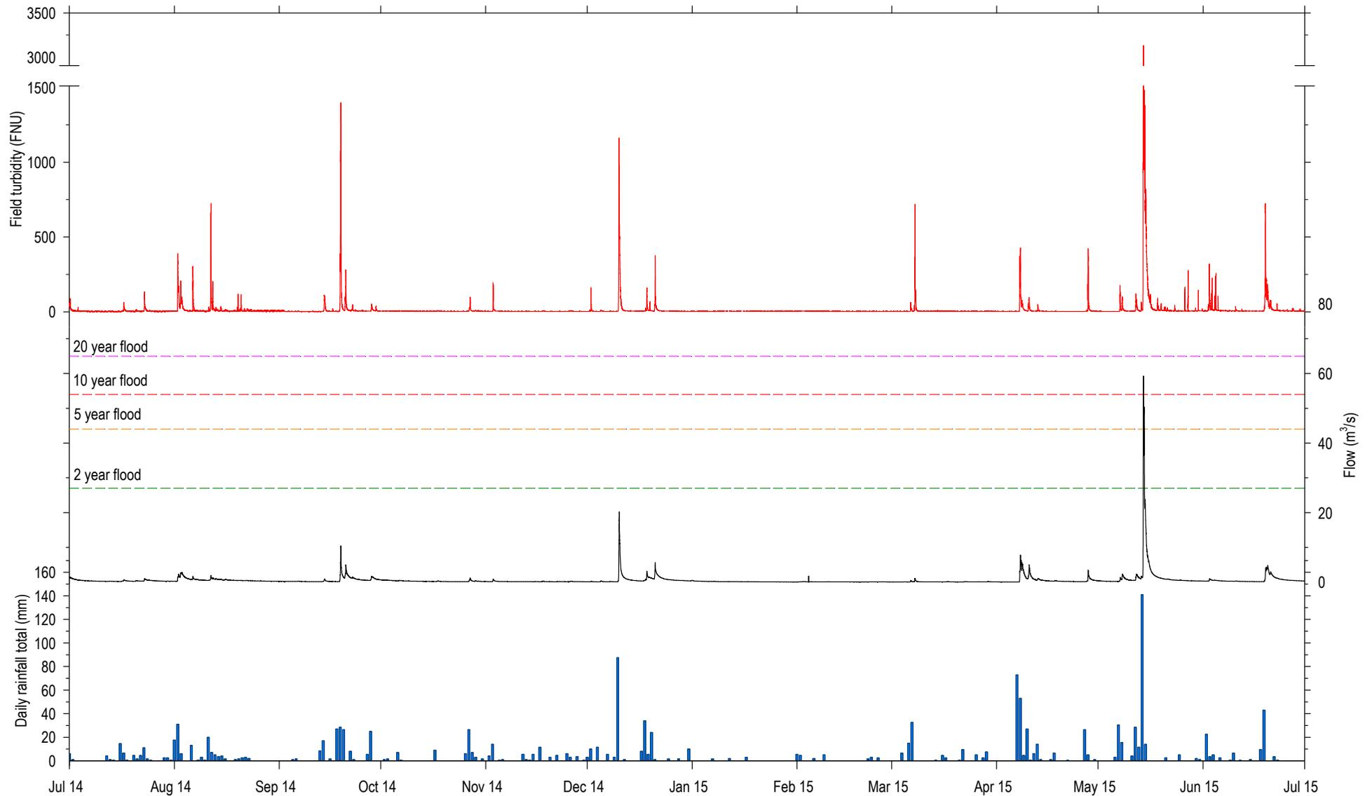
**Figure 3.6: Plots of (continuous) turbidity and flow at the Horokiri Stream monitoring site and total daily rainfall at Battle Hill Park between 1 July 2014 and 30 June 2015 (note the turbidity record for May 2015 includes some derived data)**
