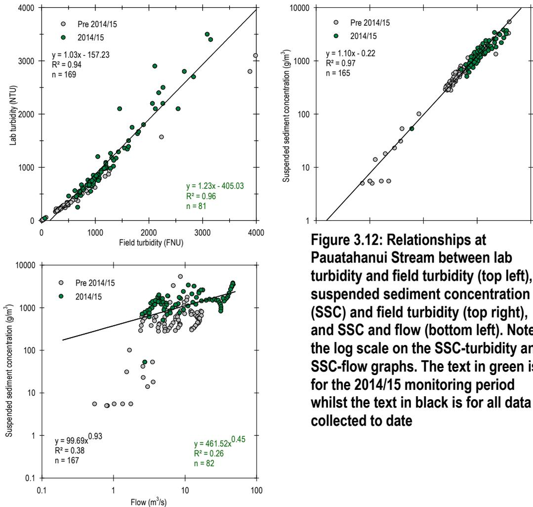
**Figure 3.12: Relationships at Pauatahanui Stream between lab turbidity and field turbidity (top left), suspended sediment concentration (SSC) and field turbidity (top right), and SSC and flow (bottom left). Note the log scale on the SSC-turbidity and SSC-flow graphs. The text in green is for the 2014/15 monitoring period whilst the text in black is for all data collected to date**
