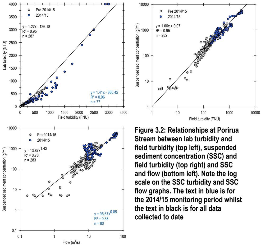
**Figure 3.2: Relationships at Porirua Stream between lab turbidity and field turbidity (top left), suspended sediment concentration (SSC) and field turbidity (top right) and SSC and flow (bottom left). Note the log scale on the SSC turbidity and SSC flow graphs. The text in blue is for the 2014/15 monitoring period whilst the text in black is for all data collected to date**
