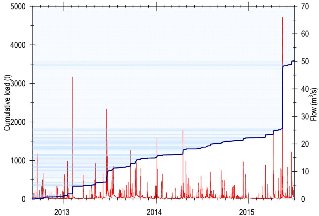
**Figure 3.4: Cumulative sediment load (blue line) versus stream flow (red line) in the Porirua Stream at Town Centre from 29 August 2012 to 30 June 2015**
