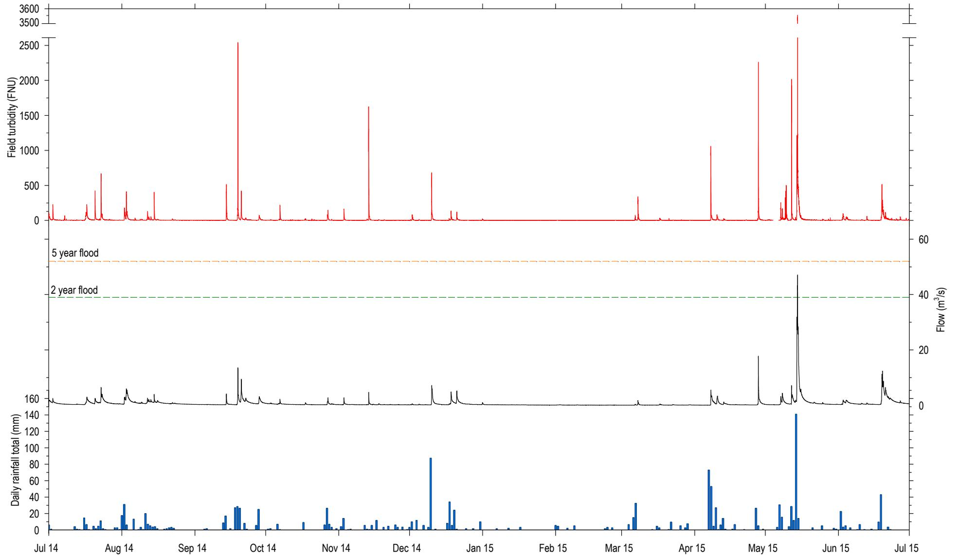
**Figure 3.11: Plots of (continuous) turbidity and flow at the Pauatahanui Stream monitoring site and total daily rainfall at Battle Hill Park between 1 July 2014 and 30 June 2015**
