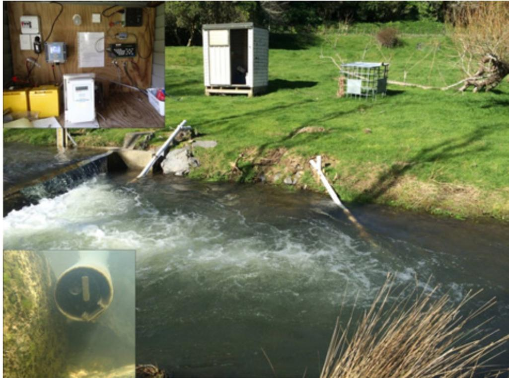
**Figure 2.3: Horokiri Stream at Snodgrass site with insets of the SC-200 control unit and logger setup (top left), and primary in-stream turbidity sensor (bottom left inset and pipe near weir). The back-up turbidity sensor can be seen (approximately 3 m) downstream of weir**
