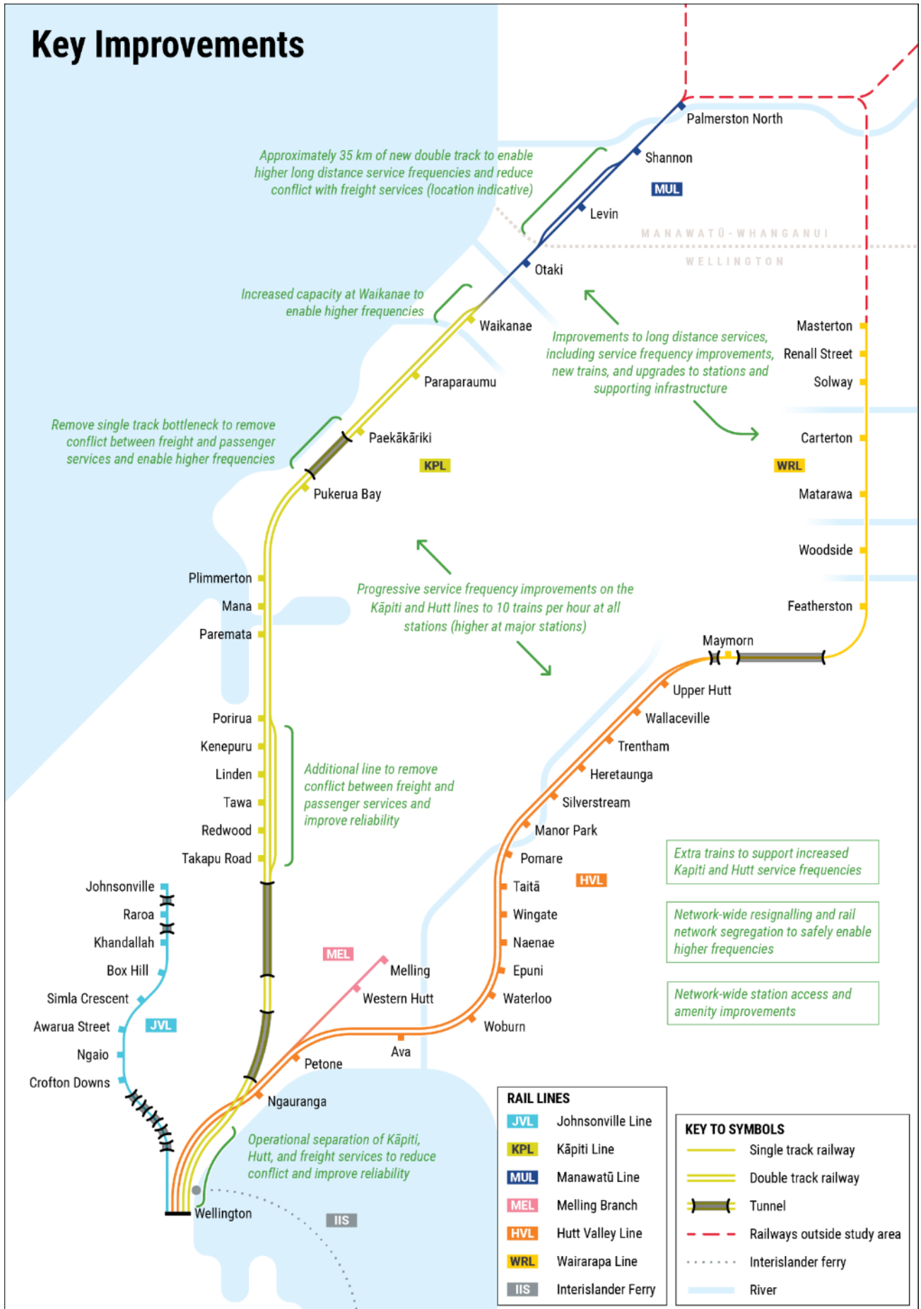
Figure 17: Planned improvements to rail infrastructure
