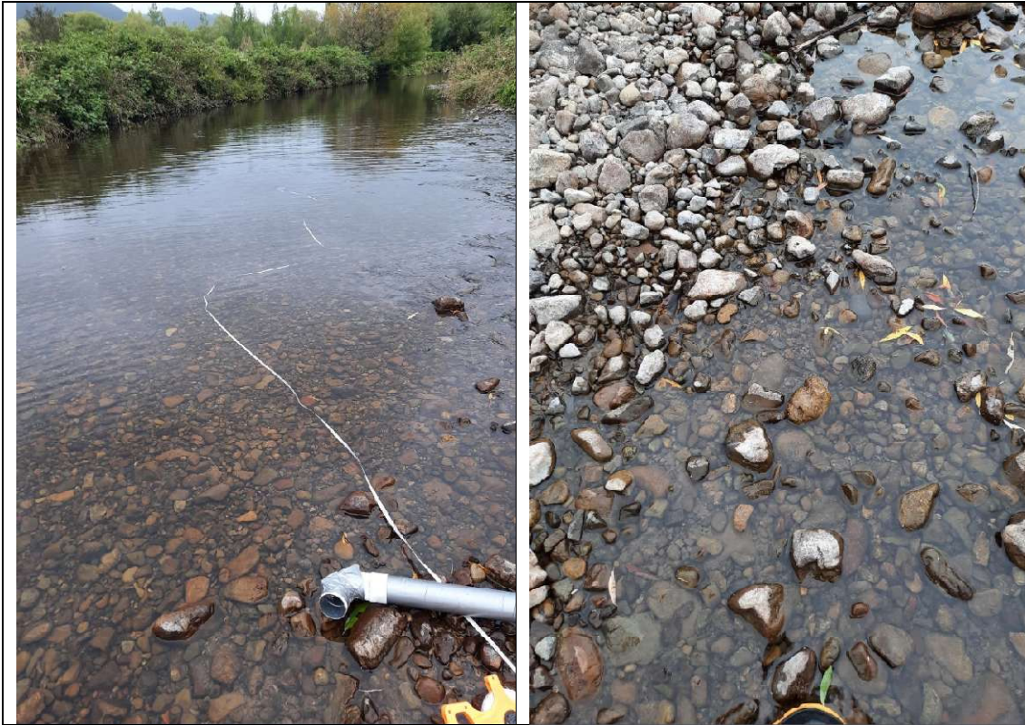
Caption for above: Alternative periscope used at sampling point just above confluence with Black Stream. 111c Mangaroa Valley Road. Photo date 29 Jan 2025
