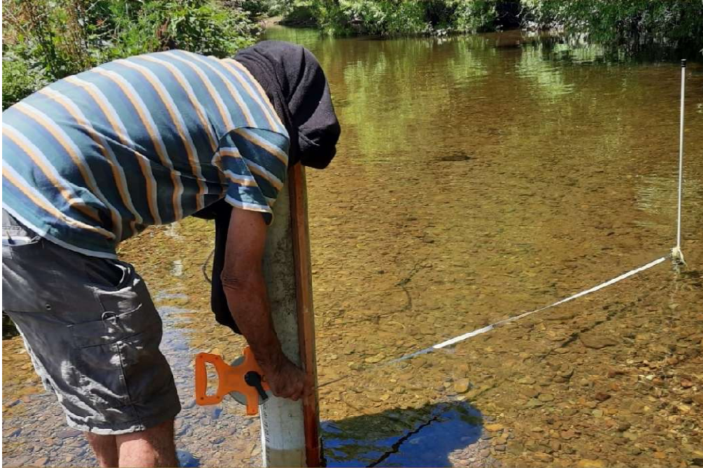
Caption. Periscope and tape measure to measure black disc visibility at Mangaroa River at intersection of Mangaroa Valley Road and Whitemans Valley Rd (above confluence with Black Stream). Larger size black spots were used in subsequent work, as defined in the official method.
