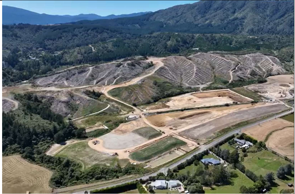
Caption: Both branches of Blaikies stream drain the Maymorn Farm Subdivision. Sediment pond in foreground. (Photo obtained by screen capture of promotional video)
